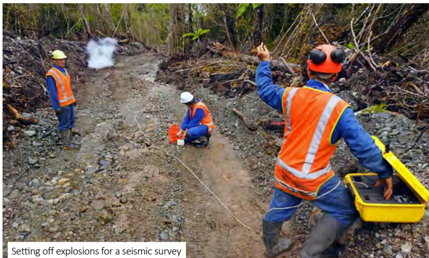
Setting off explosions for a seismic survey
